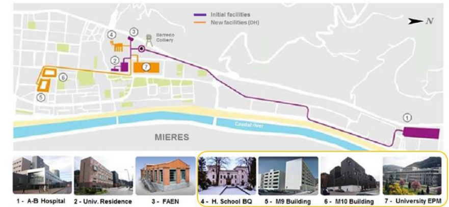
Figure 52: Map of Mieres geothermal facilities, including those of the DH system (in orange) (source: Hunosa)
